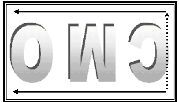
RPFI = high: display with 180degree rotation
