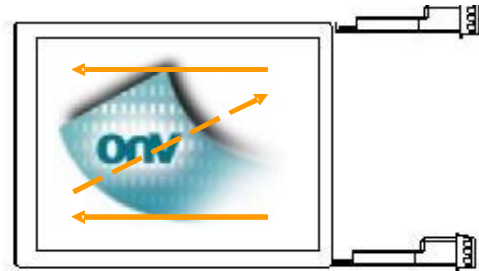
Fig. 2 Reverse scan (Pin19 = High)
