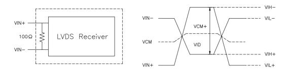
VID = VIN<sub>+</sub> - VIN<sub>-</sub>, VCM = | VCM<sub>+</sub>-VCM<sub>-</sub> | , VID = | VID<sub>+</sub>-VID<sub>-</sub> | , VID+ = | VIH<sub>+</sub>-VIH<sub>-</sub> | , VID- = | VIL<sub>+</sub>-VIL<sub>-</sub> | , VCM =(VIN<sub>+</sub>+VIN<sub>-</sub>)/2, VCM+=(VIH<sub>+</sub>+VIH<sub>-</sub>)/2, VCM<sub>-</sub> =(VIL<sub>+</sub>+VIL<sub>-</sub>)/2
