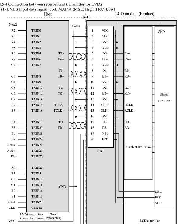
Note1: Recommended transmitter. See the data sheet for DS90C383 (Texas Instruments).
