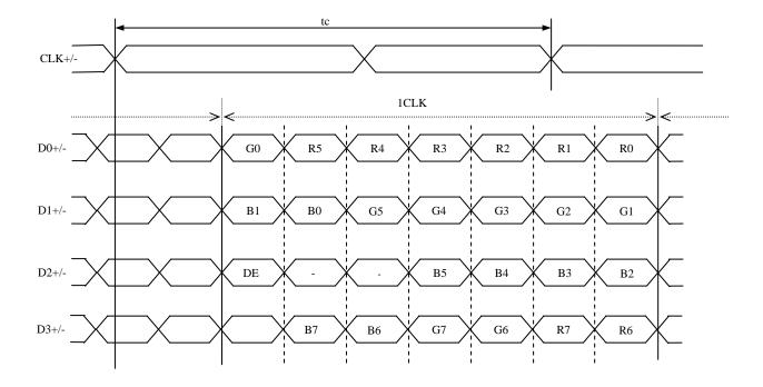
(3) LVDS Input data signal: 6bit (MSL: High, FRC: High or Open)
