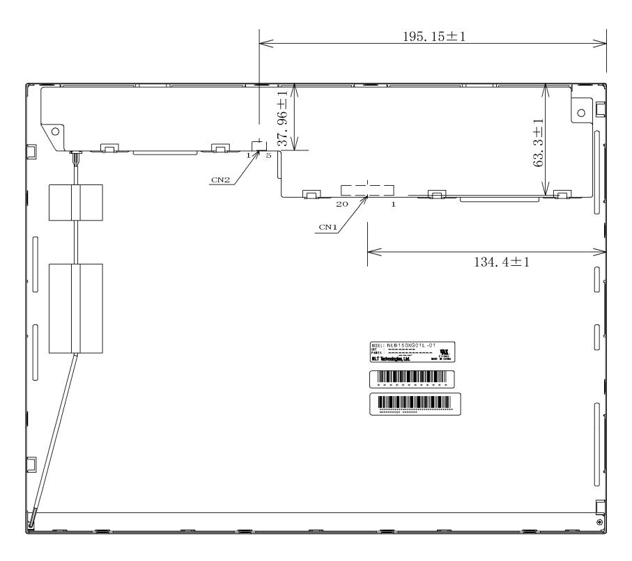
Note1: The torque for product mounting screws must never exceed  $0.392N \cdot m$ . And the length of product mounting screws must be  $\leq 4.5$  mm.
