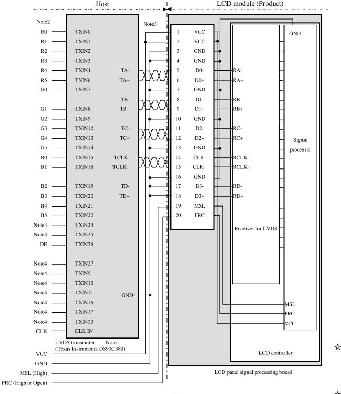
Note1: Recommended transmitter. See the data sheet for DS90C383 (Texas Instruments).
